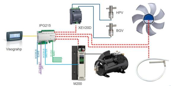
Figure 32 : Control scheme of OME
