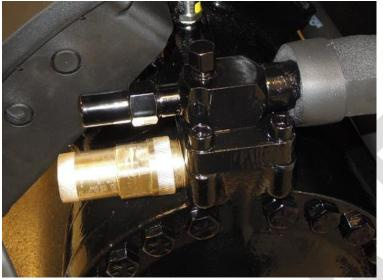
Figure 23: Low side pressure relief valve
