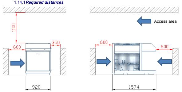
Figure 27: Fixing dimensions and distances are in mm
