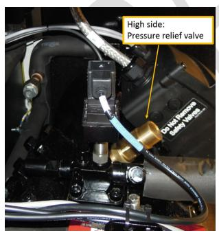
Figure 19: High side pressure relief valve
