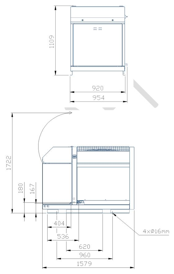
Figure 9: Dimensions of models OME-4MTL-09X, OME-4MTL-07X and OME-4MTL-05X
