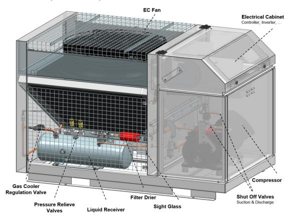
Figure 6 : Main components OME-Unit
